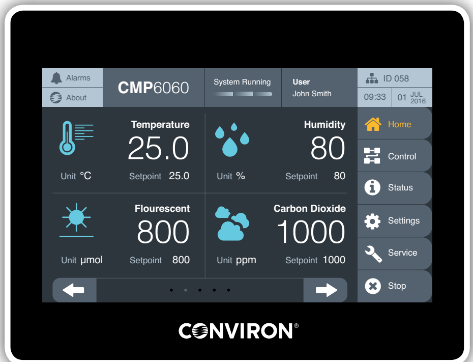
CMP6060 home screen provides an easy-viewing dashboard for set points and actual conditions and quick access to other control features.
